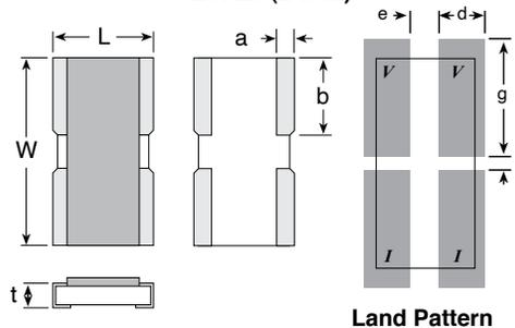
Note that LVK25 has a vertical orientation with the current flow along the short edge of the resistor.
