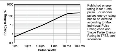
Although Ohmite's TFSS Series resistors have been specially designed and developed to absorb much more energy than standard resistors, pulses and transients require special consideration since they cause an instantaneous temperature rise in the resistor film. This application note can guide you through these considerations.
