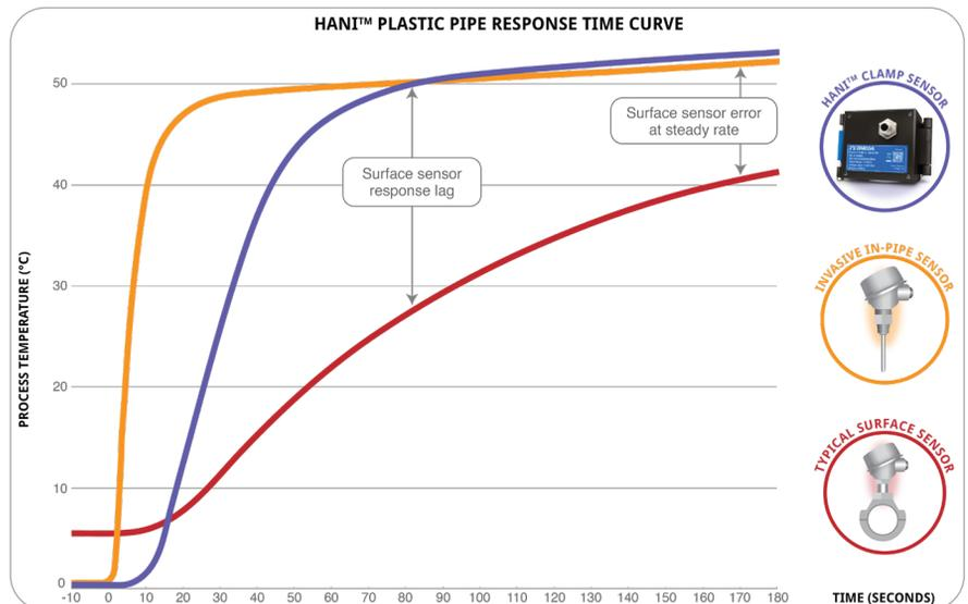
1.  $\tau_{63}$  is the time constant or response time required to reach 63.2% of the final value after an instantaneous temperature change.  $\tau_{90}$  is the response time required to reach 90% of the final value after an instantaneous temperature change.
