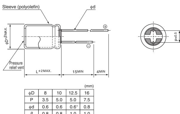
\* In case L > 25 for the φ12.5 dia. unit, lead dia. φ d = 0.8mm.
