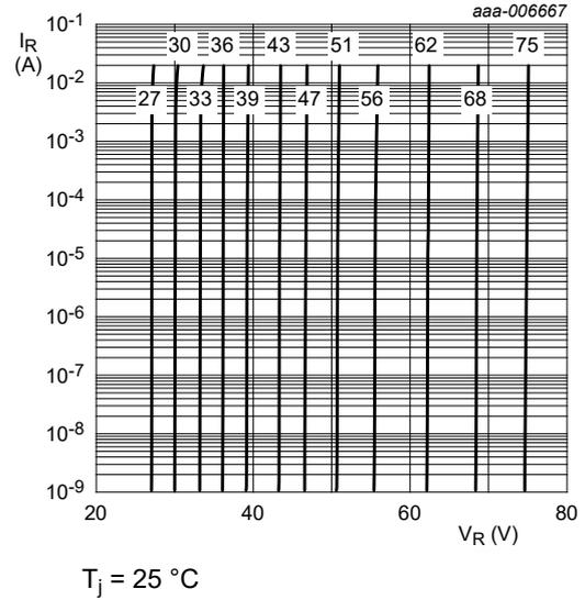
Fig. 10. Reverse current as a function of reverse voltage; typical values (MM3Z27VT1G to 75VT1G)
