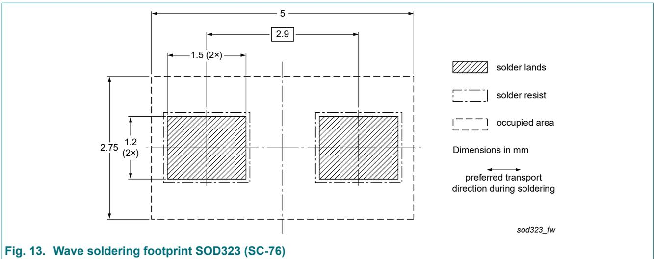
Fig. 13. Wave soldering footprint SOD323 (SC-76)
