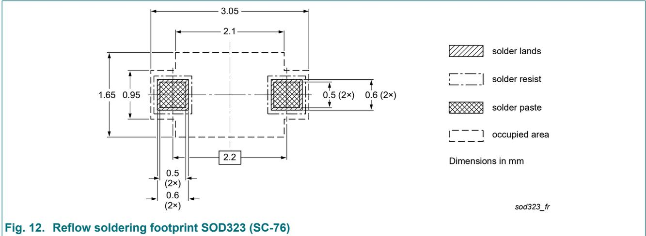
Fig. 12. Reflow soldering footprint SOD323 (SC-76)
