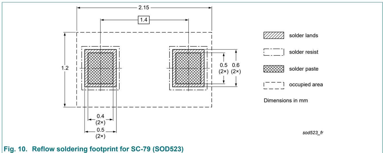
Fig. 10. Reflow soldering footprint for SC-79 (SOD523)
