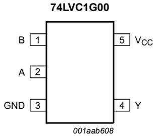
Fig. 4. Pin configuration SOT353-1 (TSSOP5) and SOT753 (SC-74A)
