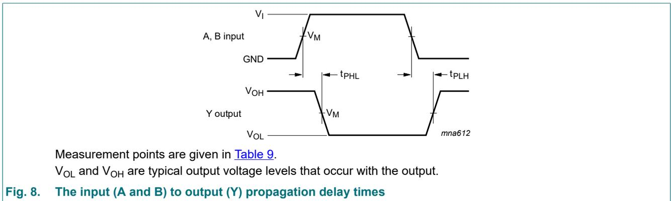
**Fig. 8. The input (A and B) to output (Y) propagation delay times**
