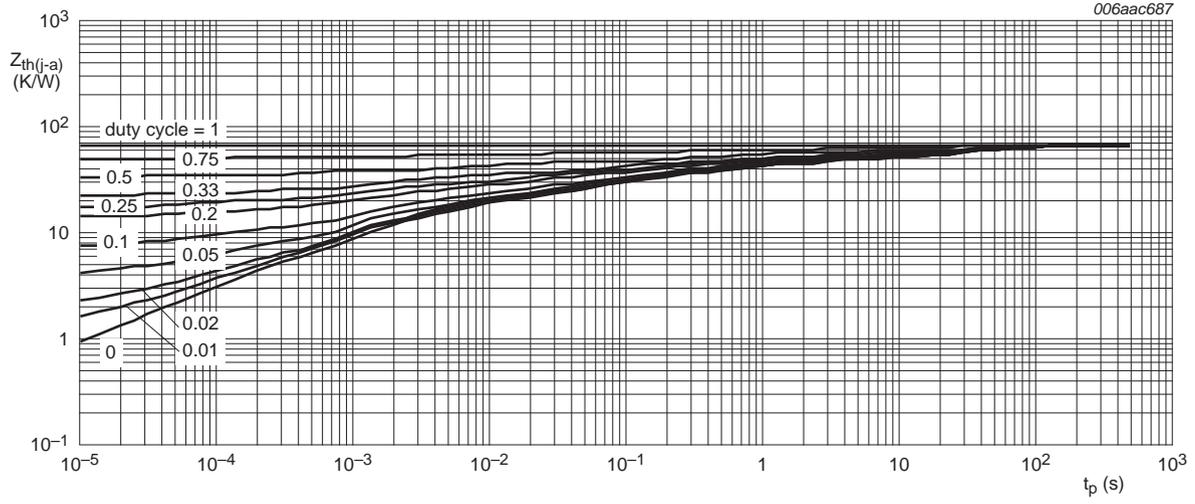
FR4 PCB, 4-layer copper, mounting pad for collector 1 cm<sup>2</sup>
