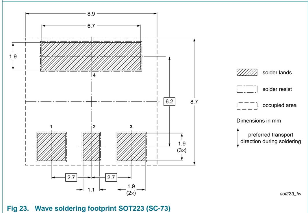
**Fig 23. Wave soldering footprint SOT223 (SC-73)**
