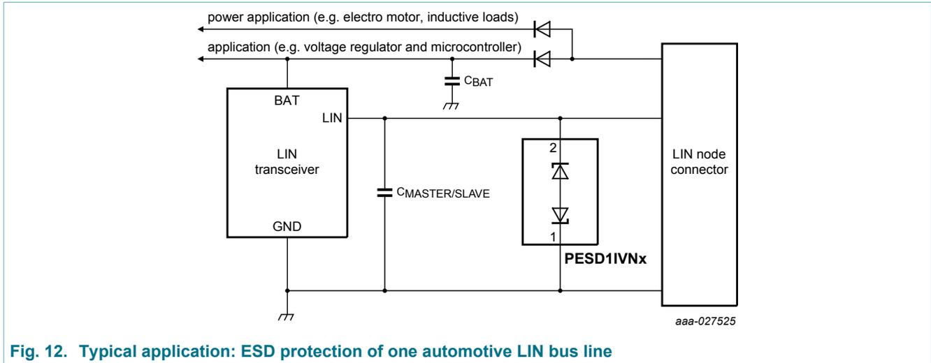
Fig. 12. Typical application: ESD protection of one automotive LIN bus line
