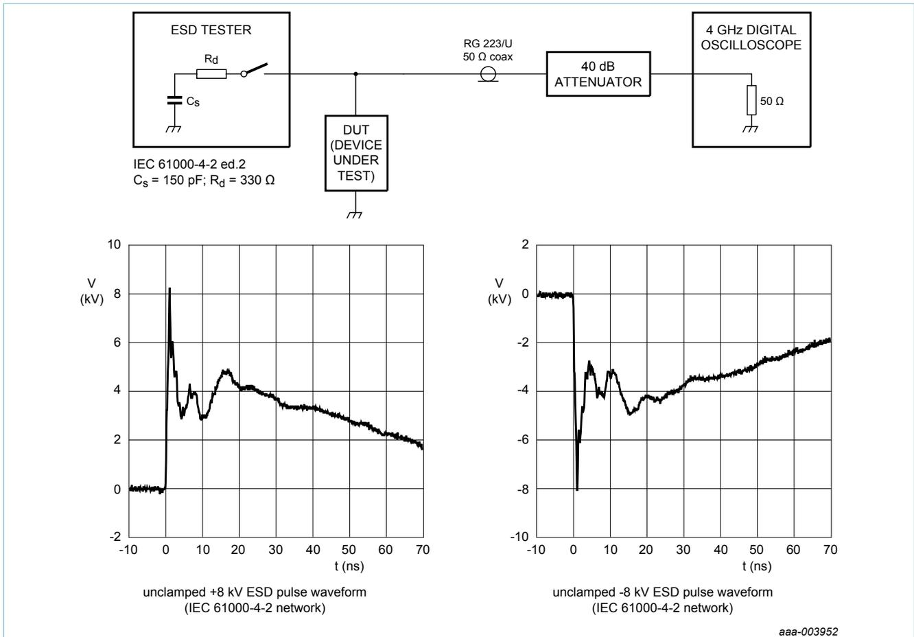
Fig. 9. ESD clamping test setup and waveforms
