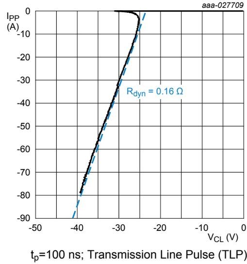
Fig. 6. Negative clamping voltage (TLP); typical values
