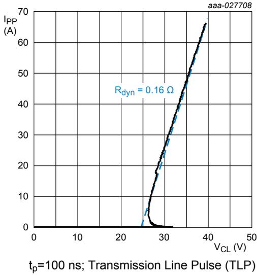
Fig. 5. Positive clamping voltage (TLP); typical values
