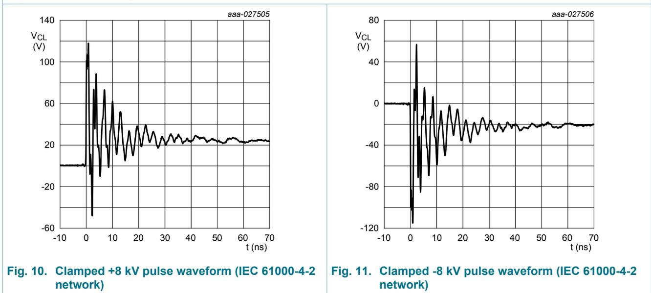
Fig. 10. Clamped +8 kV pulse waveform (IEC 61000-4-2 network)
