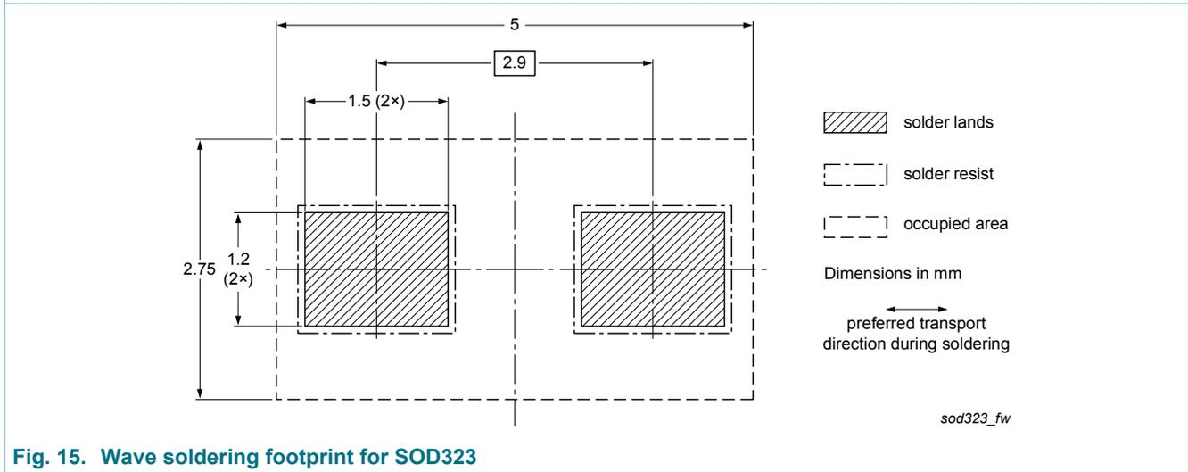
Fig. 15. Wave soldering footprint for SOD323
