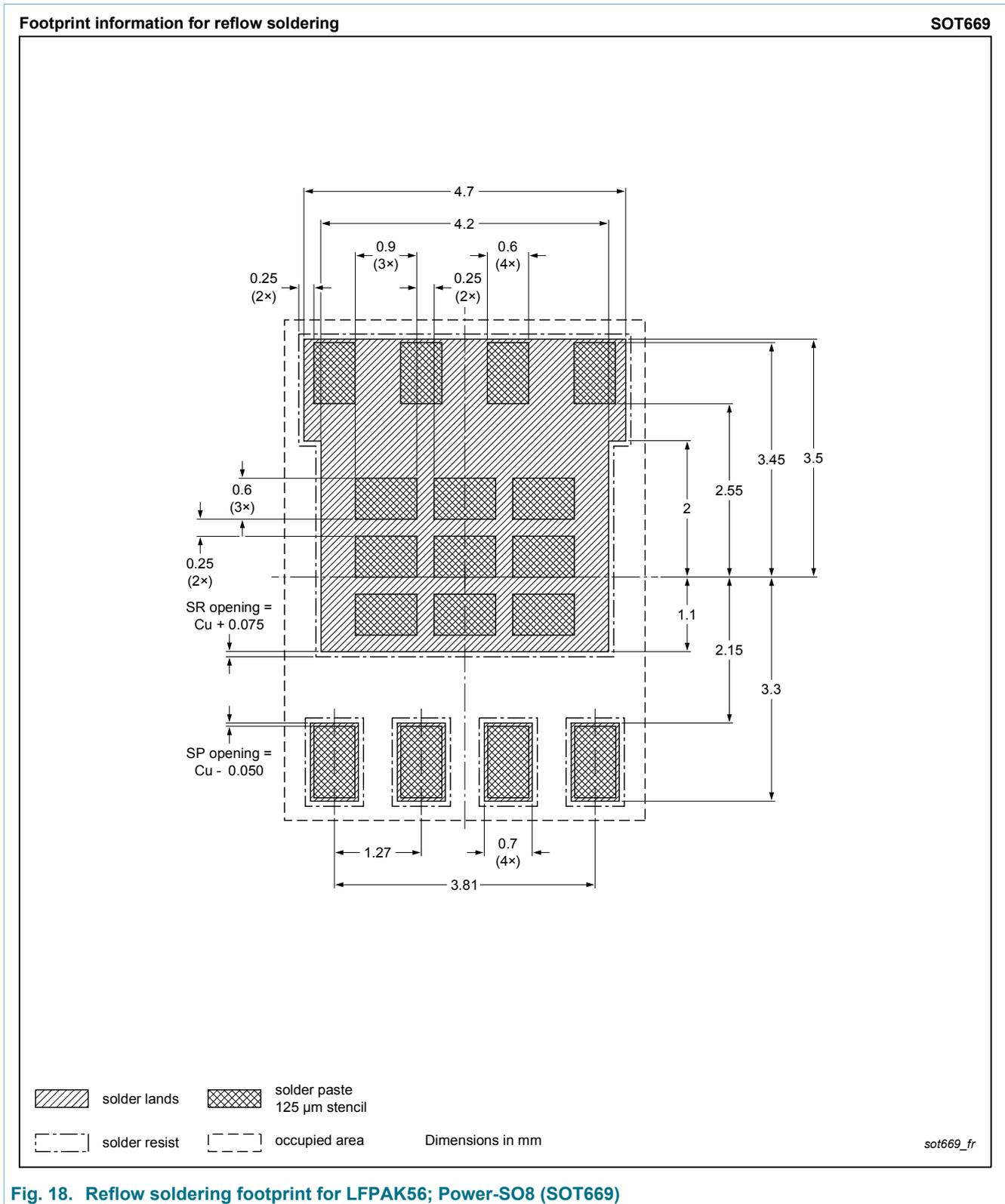
**Fig. 18. Reflow soldering footprint for LPAK56; Power-SO8 (SOT669)**
