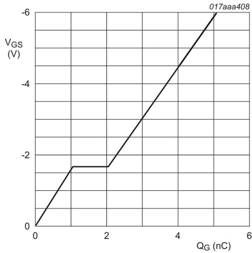
$I_D = -3.3$  A;  $V_{DS} = -10$  V;  $T_{amb} = 25$  °C
