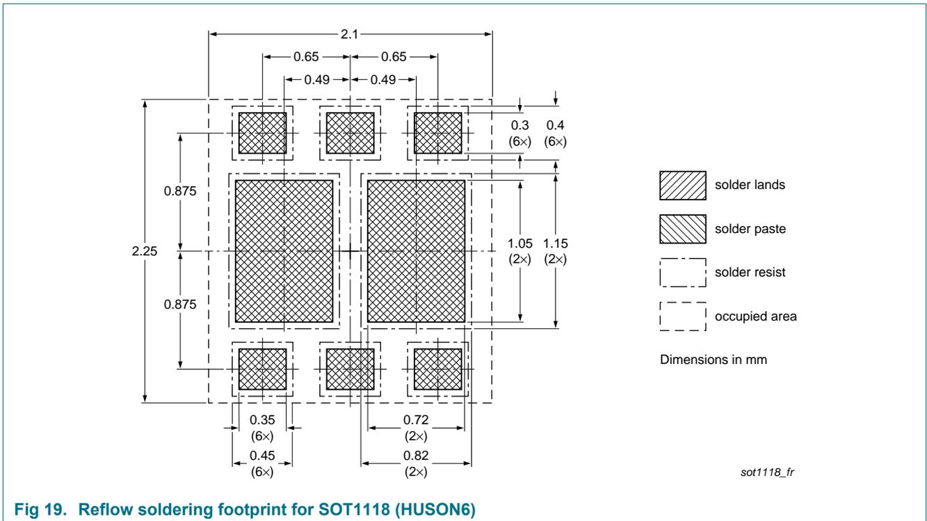
Fig 19. Reflow soldering footprint for SOT1118 (HUSON6)
