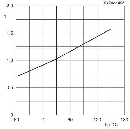
$$a = \frac{R_{DSon}}{R_{DSon(25^\circ\text{C})}}$$
