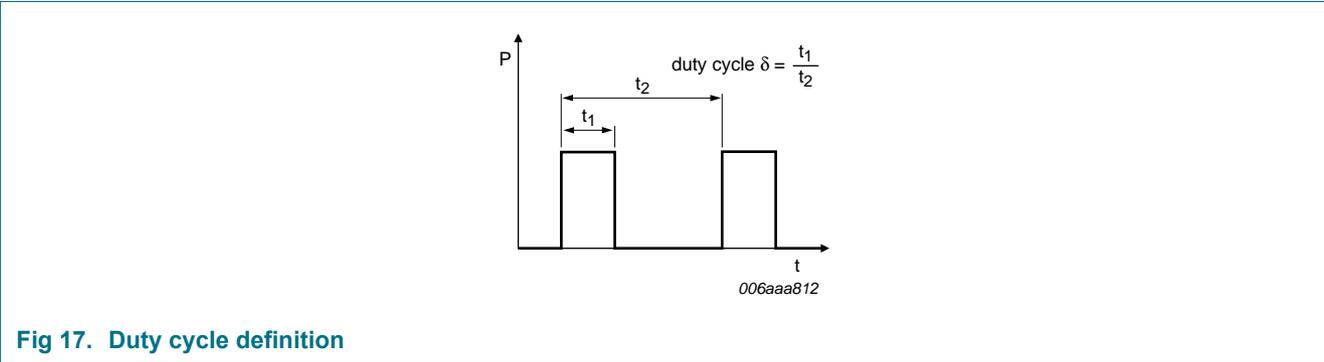
Fig 17. Duty cycle definition
