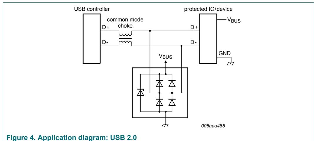
Figure 4. Application diagram: USB 2.0
