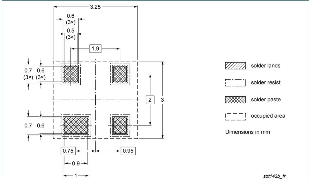
Figure 6. Reflow soldering footprint SOT143B
