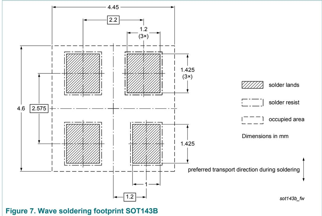
Figure 7. Wave soldering footprint SOT143B
