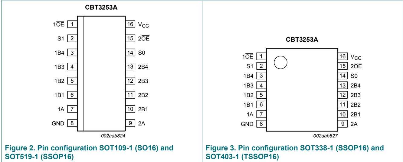
Figure 2. Pin configuration SOT109-1 (SO16) and SOT519-1 (SSOP16)
