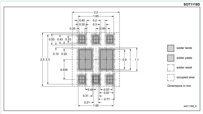
Fig. 21. Reflow soldering footprint for DFN2020D-6 (SOT1118D)
