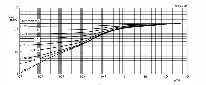
FR4 PCB 35 µm, mounting pad for collector 1 cm<sup>2</sup>
