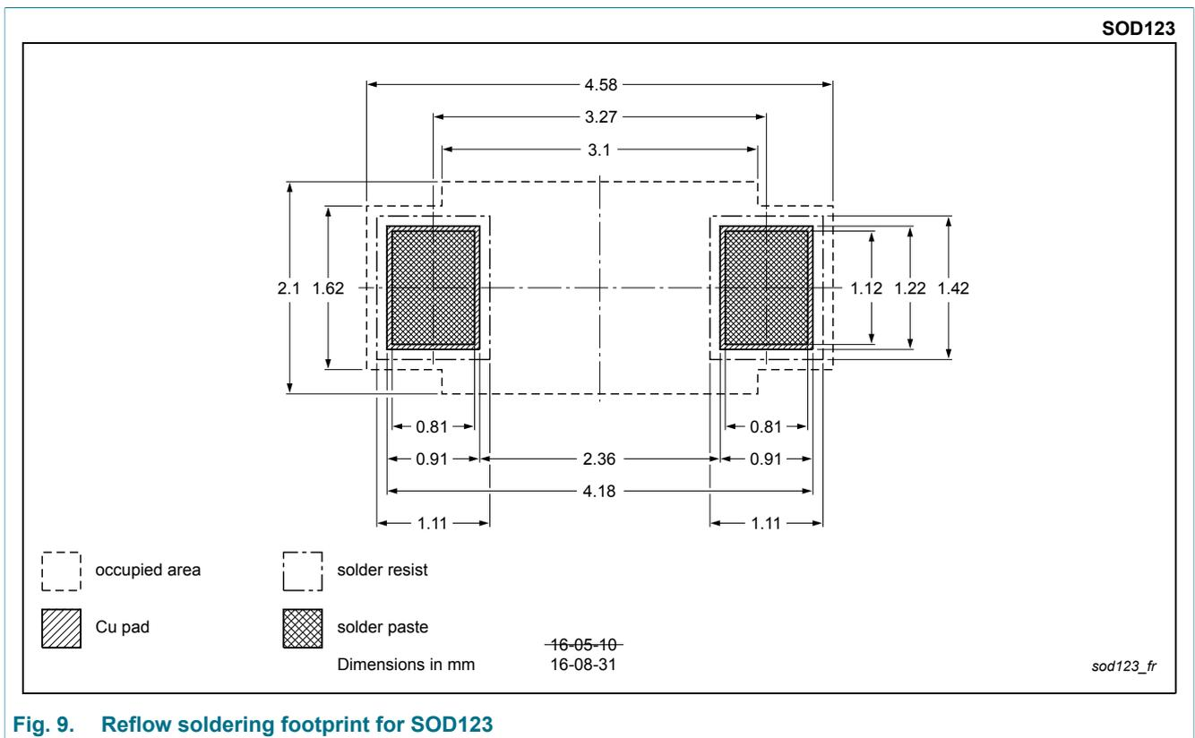
Fig. 9. Reflow soldering footprint for SOD123
