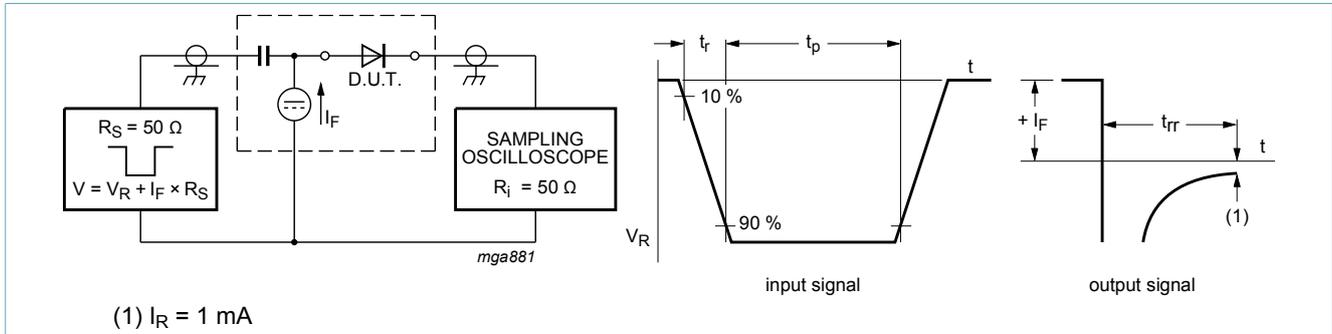
Fig. 9. Reverse recovery time test circuit and waveforms
