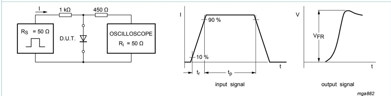
Fig. 10. Forward recovery voltage test circuit and waveforms
