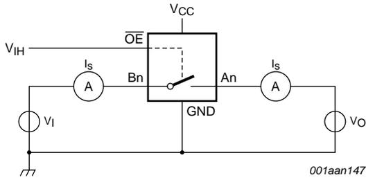
$V_I = V_{CC}$  or GND and  $V_O =$  GND or  $V_{CC}$ .
