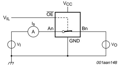
$V_I = V_{CC}$  or GND and  $V_O =$  open circuit.
