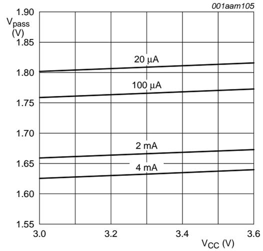
**Fig 10. Pass voltage versus supply voltage; T<sub>amb</sub> = 0 °C (typical)**
