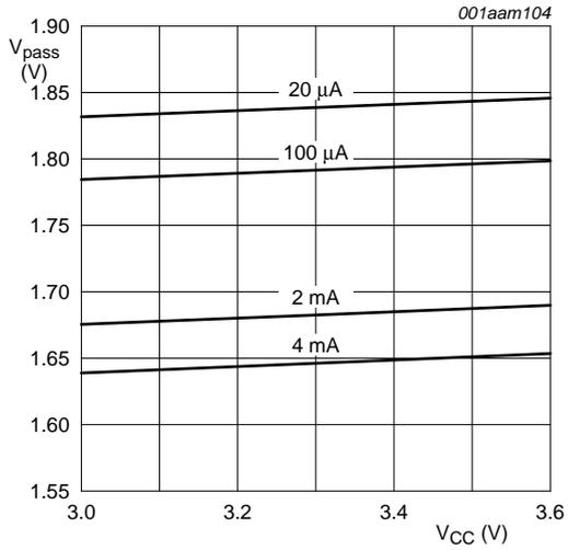
**Fig 9. Pass voltage versus supply voltage; T<sub>amb</sub> = 25 °C (typical)**
