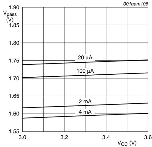
**Fig 11. Pass voltage versus supply voltage; T<sub>amb</sub> = -40 °C (typical)**
