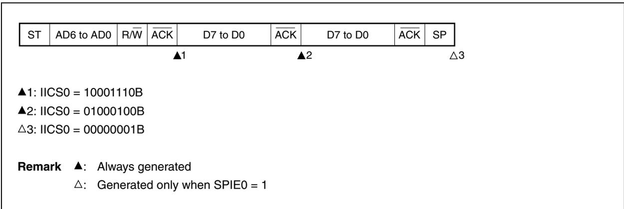
(d) When loss occurs due to restart condition during data transfer
