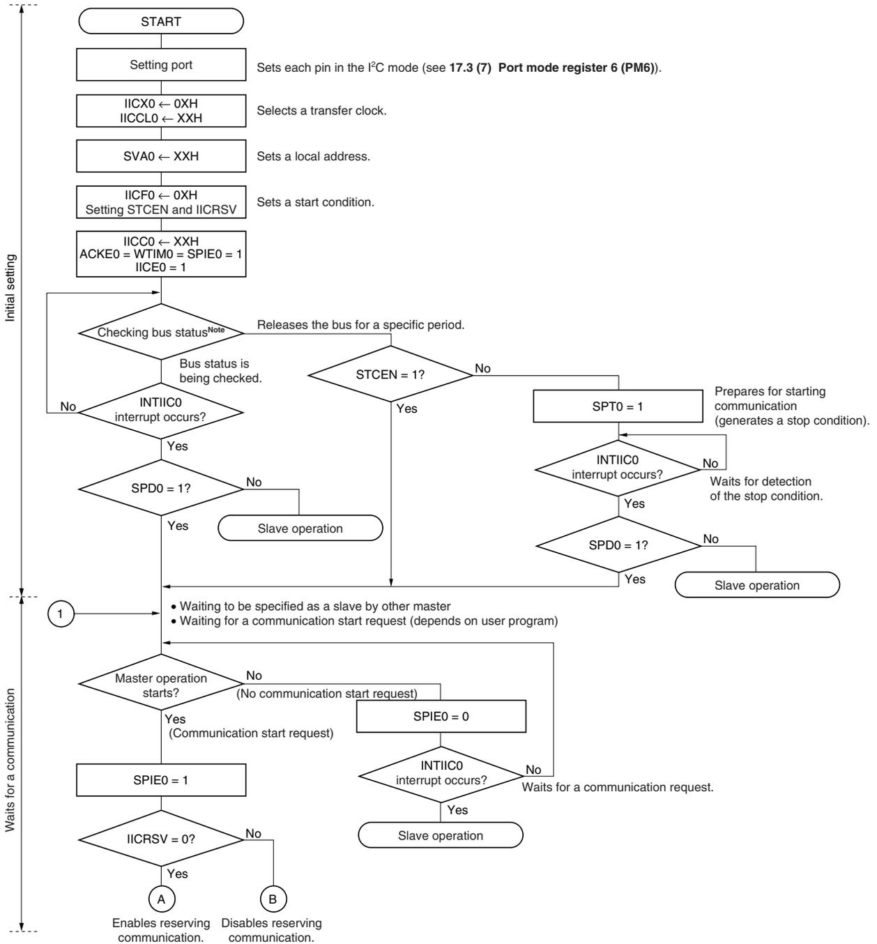
**Note** Confirm that the bus is released (CLD0 bit = 1, DAD0 bit = 1) for a specific period (for example, for a period of one frame). If the SDA0 pin is constantly at low level, decide whether to release the I<sup>2</sup>C bus (SCL0 and SDA0 pins = high level) in conformance with the specifications of the product that is communicating.
