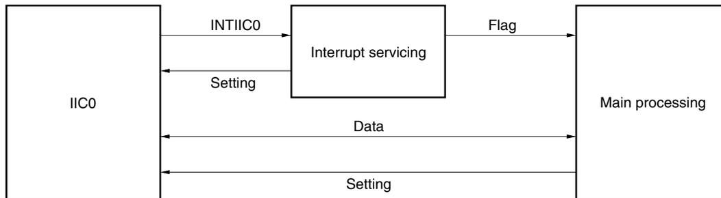
Therefore, data communication processing is performed by preparing the following three flags and passing them to the main processing instead of INTIIC0.
