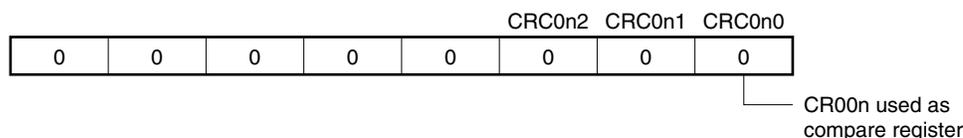
**(c) 16-bit timer output control register 0n (TOC0n)**
