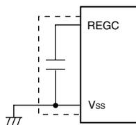
**★ Caution** Keep the wiring length as short as possible for the broken-line part in the above figure.
