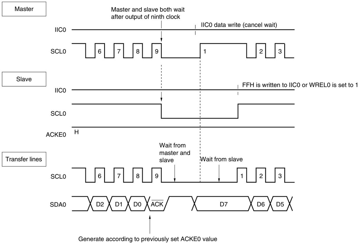
**Remark** ACKE0: Bit 2 of IIC control register 0 (IICC0)
