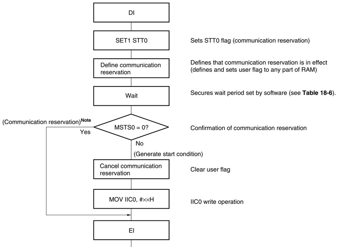
**Note** The communication reservation operation executes a write to IIC shift register 0 (IIC0) when a stop condition interrupt request occurs.
