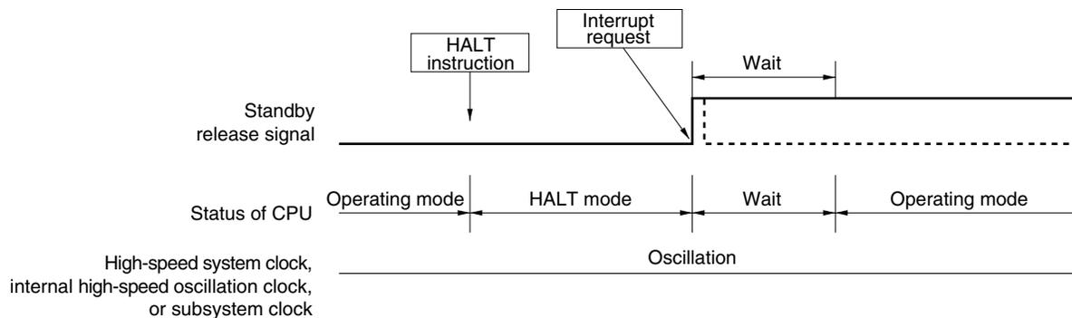
**Remarks 1.** The broken lines indicate the case when the interrupt request which has released the standby mode is acknowledged.
