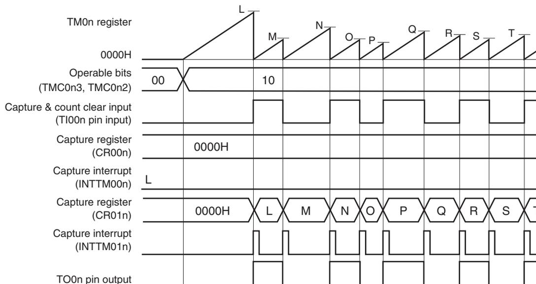
This is an application example where the count value is captured to CR01n, TM0n is cleared, and the TO0n pin output is inverted when the rising or falling edge of the TI00n pin is detected.
