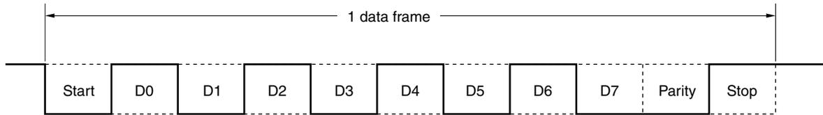
2. Data length: 8 bits, MSB first, Parity: Even parity, Stop bit: 1 bit, Communication data: 55H
