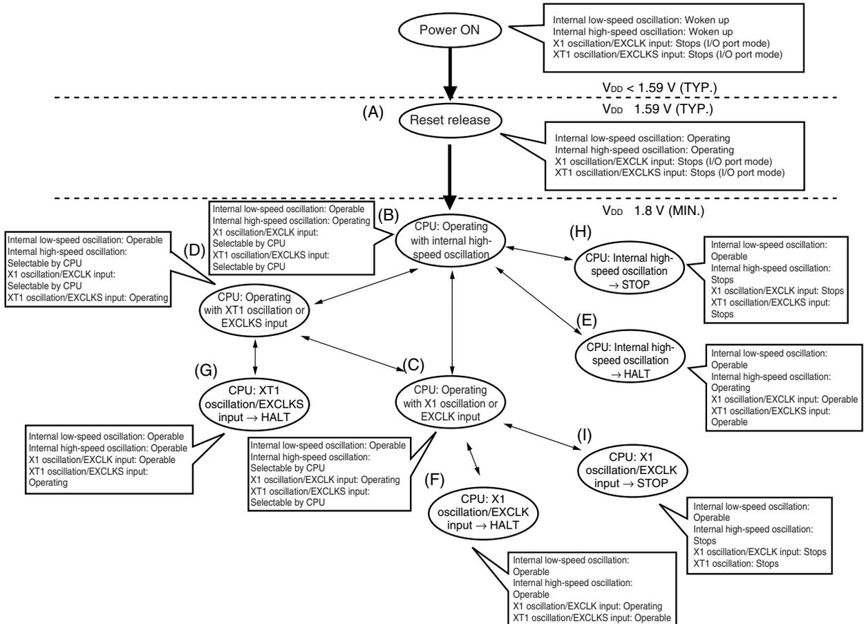
★ **Remark** In the 2.7 V/1.59 V POC mode (option byte: POCMODE = 1), the CPU clock status changes to (A) in the above figure when the supply voltage exceeds 2.7 V (TYP.), and to (B) after reset processing (20  $\mu\text{s}$  (TYP.)).
