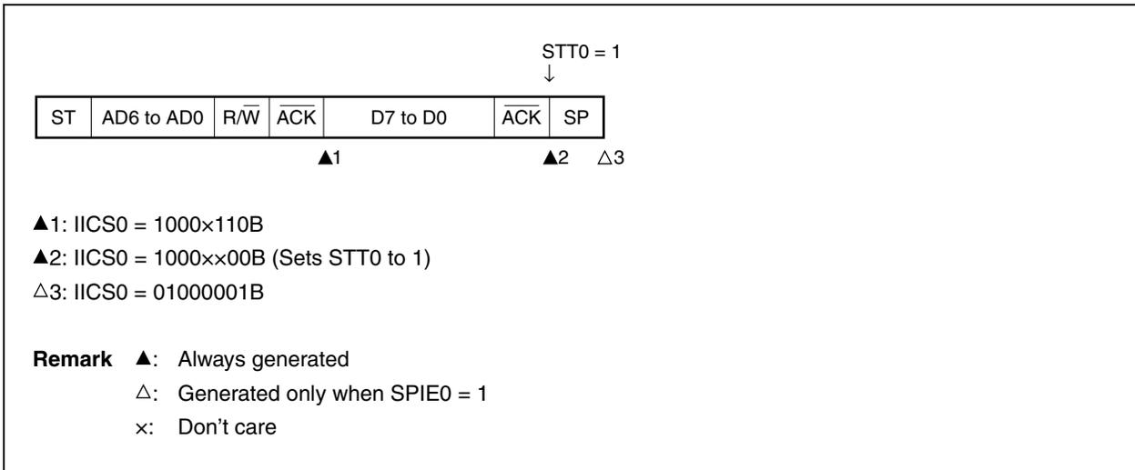
(h) When arbitration loss occurs due to low-level data when attempting to generate a stop condition
