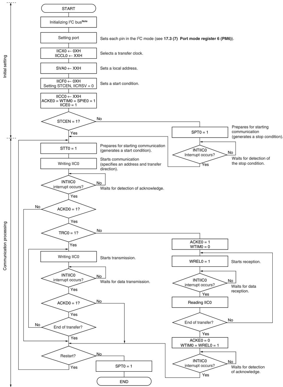
**Note** Release (SCL0 and SDA0 pins = high level) the I<sup>2</sup>C bus in conformance with the specifications of the product that is communicating. If EEPROM is outputting a low level to the SDA0 pin, for example, set the SCL0 pin in the output port mode, and output a clock pulse from the output port until the SDA0 pin is constantly at high level.
