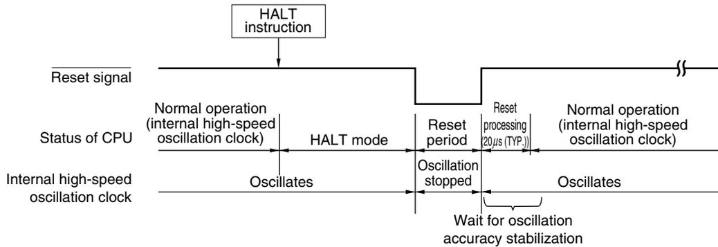
**(3) When subsystem clock is used as CPU clock**
