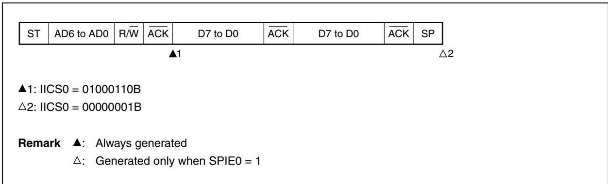
(b) When arbitration loss occurs during transmission of extension code
