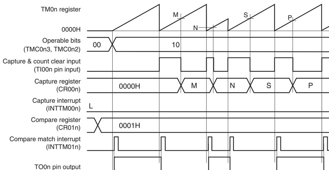
This is an application example where the output level of the TO0n pin is to be inverted when the count value has been captured & cleared.
