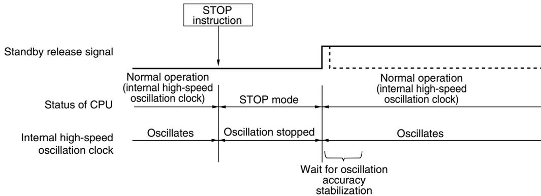
**Remark** The broken lines indicate the case when the interrupt request that has released the standby mode is acknowledged.
