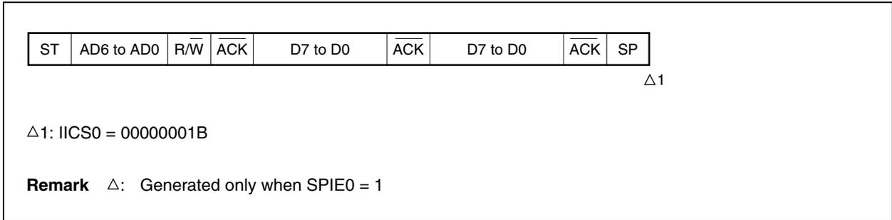
**(5) Arbitration loss operation (operation as slave after arbitration loss)**
