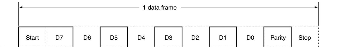
4. Data length: 7 bits, LSB first, Parity: Odd parity, Stop bit: 2 bits, Communication data: 36H
