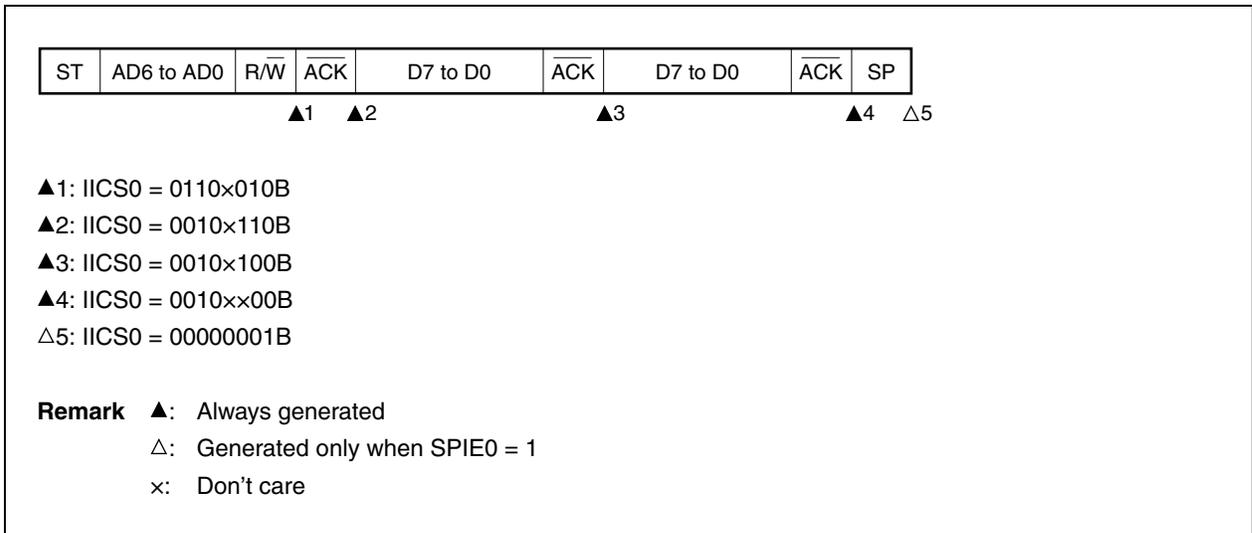
(6) Operation when arbitration loss occurs (no communication after arbitration loss)
