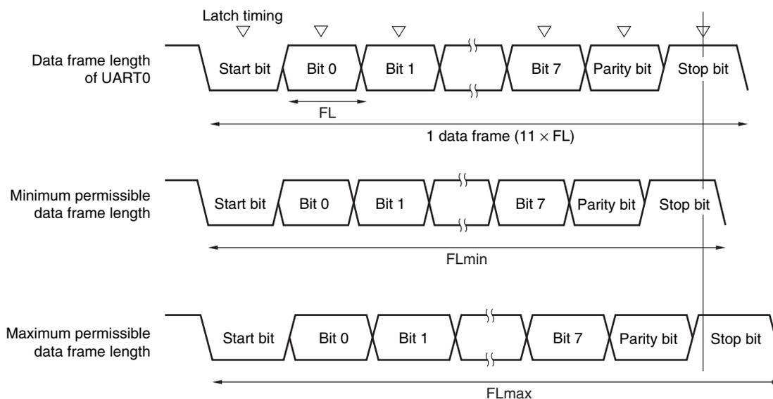
As shown in Figure 14-12, the latch timing of the receive data is determined by the counter set by baud rate generator control register 0 (BRGC0) after the start bit has been detected. If the last data (stop bit) meets this latch timing, the data can be correctly received.
