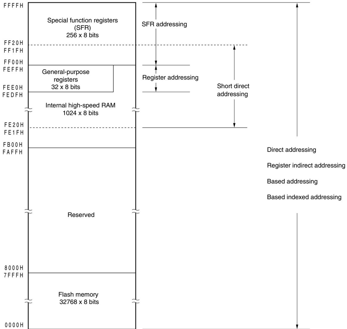
Figure 3-12. Correspondence Between Data Memory and Addressing ( $\mu$ PD78F0534)
