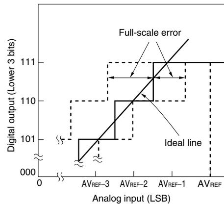
**Figure 13-18. Integral Linearity Error**
