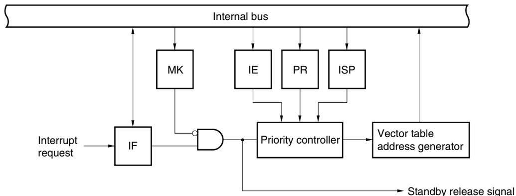
(B) External maskable interrupt (INTP0 to INTP7)
