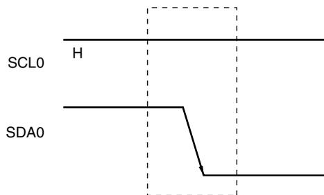
A start condition is output when bit 1 (STT0) of IIC control register 0 (IICC0) is set (to 1) after a stop condition has been detected (SPD0: Bit 0 = 1 in IIC status register 0 (IICS0)). When a start condition is detected, bit 1 (STD0) of IICS0 is set (to 1).
