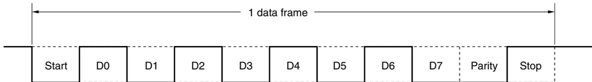
2. Data length: 7 bits, Parity: Odd parity, Stop bit: 2 bits, Communication data: 36H
