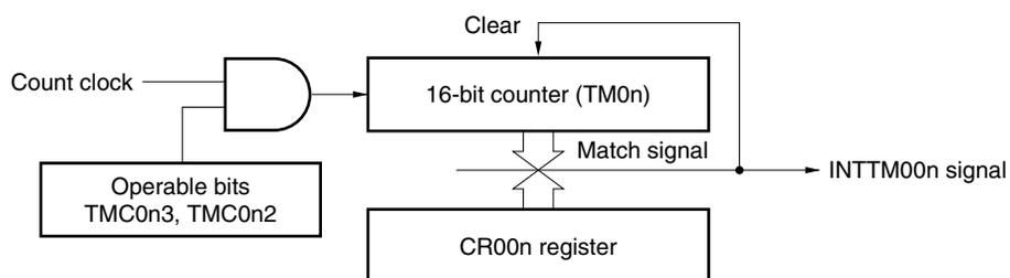
**Figure 7-17. Basic Timing Example of Interval Timer Operation**
