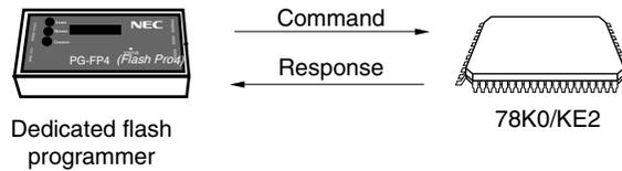
The flash memory control commands of the 78K0/KE2 are listed in the table below. All these commands are issued from the programmer and the 78K0/KE2 perform processing corresponding to the respective commands.
