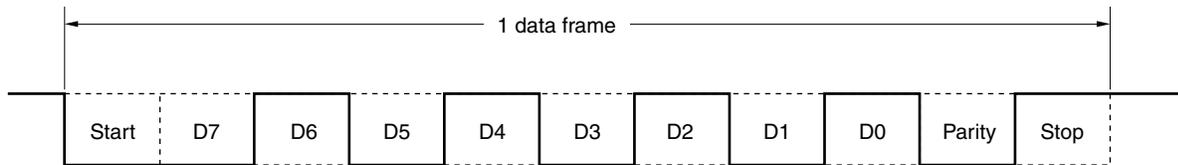
3. Data length: 8 bits, MSB first, Parity: Even parity, Stop bit: 1 bit, Communication data: 55H, Tx/D6 pin inverted output
