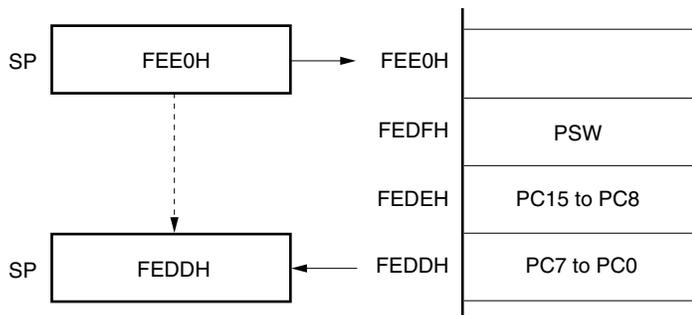
Figure 3-20. Data to Be Restored from Stack Memory
