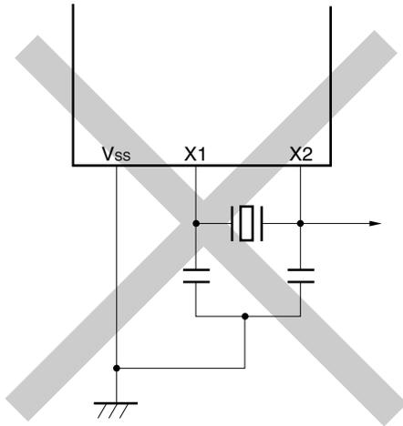
**Remark** When using the subsystem clock, replace X1 and X2 with XT1 and XT2, respectively. Also, insert resistors in series on the XT2 side.
