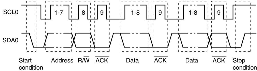
The master device generates the start condition, slave address, and stop condition.
