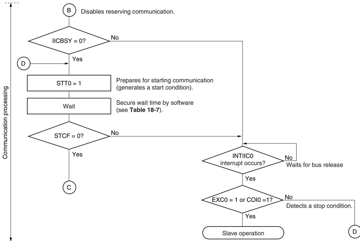
Figure 17-24. Master Operation Flowchart (Multi-Master System) (3/3)
