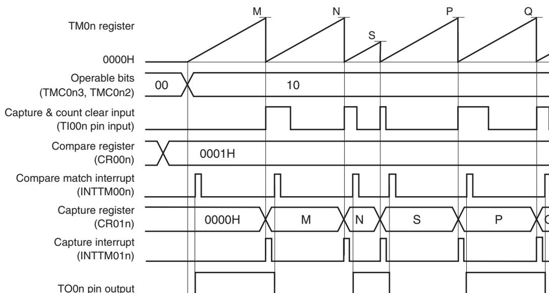
This is an application example where the output level of the TO0n pin is inverted when the count value has been captured & cleared.
