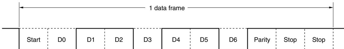
3. Data length: 8 bits, Parity: None, Stop bit: 1 bit, Communication data: 87H
