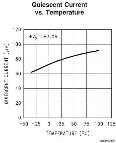
**Typical Performance Characteristics** To generate these curves the LM62 was mounted to a printed circuit board as shown in Figure 2. (Continued)
