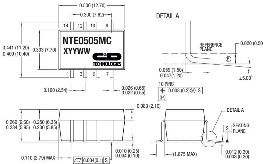
All dimensions in inches  $\pm 0.01$  (mm  $\pm 0.25$ mm). All pins on a 0.1 (2.54) pitch and within  $\pm 0.01$  (0.25) of true position.
