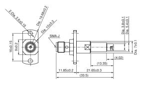
Measurement Probe for MM8130-2600/MM8430-2610 (P/N: MXHS83QE3000)
