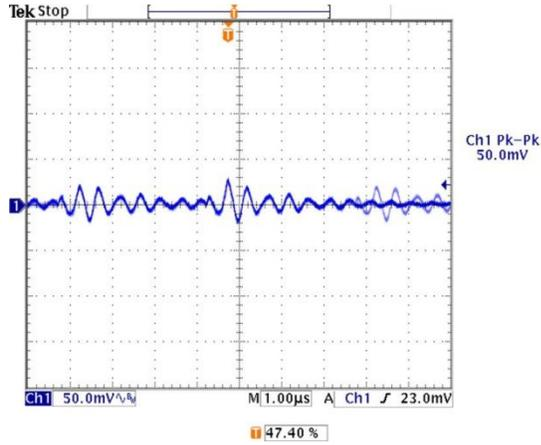
Output Ripple and Noise ( $V_{in}=24V$ ,  $V_{out}=nom.$ ,  $I_{out}=2A$ ,  $C_{load}=1\mu F$  ceramic II  $10\mu F$  tantalum,  $T_a=+25^{\circ}C.$ , ScopeBW=20MHz)
