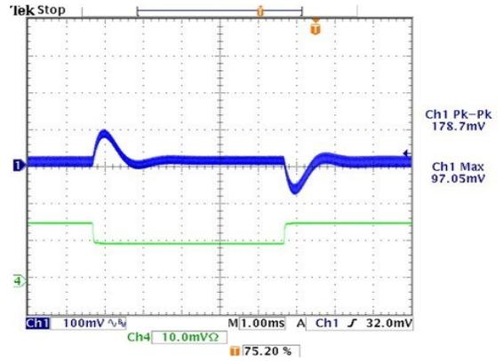
Power On Startup Delay ( $V_{in}=0$  to  $24V$ ,  $V_{out}=nom.$ ,  $I_{out}=no$  load,  $C_{load}=0\mu F$ ,  $T_a=+25^\circ C.$ , ScopeBW=20MHz) Trace 1= $V_{in}$ , Trace 2= $V_{out}$
