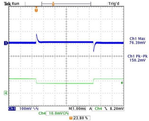
Power On Startup Delay ( $V_{in}=0$  to 24V,  $V_{out}=nom.$ ,  $I_{out}=no$  load,  $C_{load}=0\mu F$ ,  $T_a=+25^\circ C.$ , ScopeBW=20MHz) Trace 1= $V_{in}$ , Trace 2= $V_{out}$
