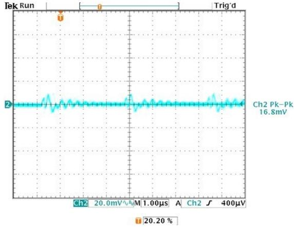
Output Ripple and Noise ( $V_{in}=24V$ ,  $V_{out}=nom.$ ,  $I_{out}=4.5A$ ,  $C_{load}=1\mu F$  ceramic II  $10\mu F$  tantalum,  $T_a=+25^{\circ}C.$ , ScopeBW=20MHz)
