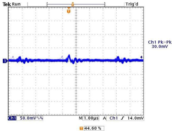
Output Ripple and Noise (Vin=24V, Vout=nom., Iout=3.3A, Cload=1μF ceramic || 10μF tantalum, Ta=+25°C., ScopeBW=20MHz)
