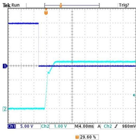
On/Off Enable Delay (Negative logic, Vin=24V, Vout=nom., Iout=15A, Cload=0 μF, Ta=+25°C., ScopeBW=20MHz) Trace 1=Enable, Trace 2=Vout
