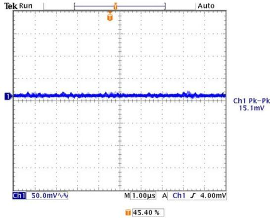
Output Ripple and Noise ( $V_{in}=24V$ ,  $V_{out}=\text{nom.}$ ,  $I_{out}=10A$ ,  $C_{load}=1\mu F$  ceramic ||  $10\mu F$  tantalum,  $T_a=+25^\circ C$ ., ScopeBW=20MHz)
