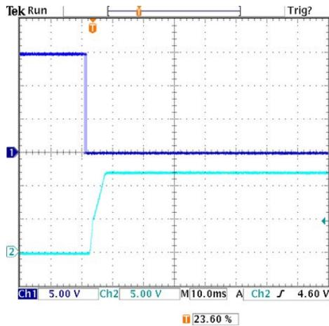
On/Off Enable Delay (Negative logic,  $V_{in}=24V$ ,  $V_{out}=nom.$ ,  $I_{out}=4.5A$ ,  $C_{load}=0\mu F$ ,  $T_a=+25^{\circ}C.$ , ScopeBW=20MHz) Trace 1=Enable, Trace 2=Vout
