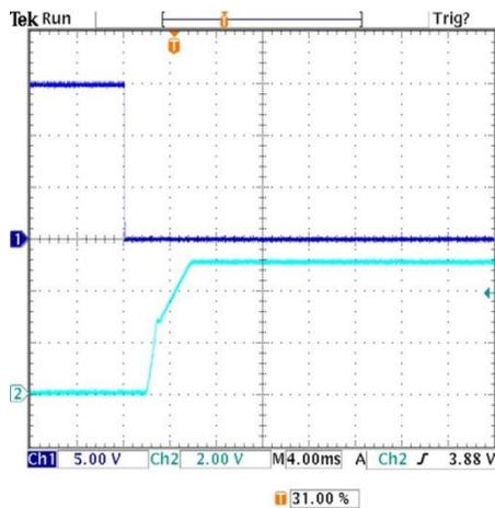
On/Off Enable Delay (Negative logic,  $V_{in}=24V$ ,  $V_{out}=\text{nom.}$ ,  $I_{out}=10A$ ,  $C_{load}=0\mu F$ ,  $T_a=+25^\circ C$ ., ScopeBW=20MHz) Trace 1=Enable, Trace 2=Vout
