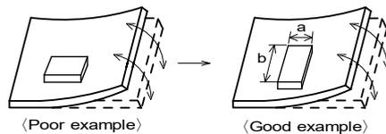
Products shall be location the sideways Direction (Length : a<b) to the mechanical Stress.
