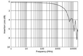
**Common Mode Insertion Loss Characteristic** (Typical Value)
