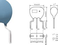
T<sup>11</sup>: 3.5±1.0 (16.00–32.99MHz) 3.0±1.0 (33.00–70.00MHz) : Frequency Marking \* : EIAJ Monthly Code (in mm) Note: This datasheet may be out of date. Please download the latest datasheet of CSTLS20M0X51-B0 from the official website of Murata Manufacturing Co., Ltd.
