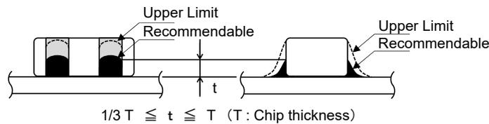
Accordingly increasing the solder volume, the mechanical stress to product is also increased. Excessive solder volume may cause the failure of mechanical or electrical performance.
