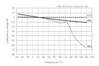
Capacitance - temperature characteristics
