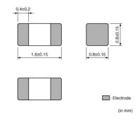
The chip ferrite beads BLM series is designed to function nearly as a resistor at noise frequencies, which greatly reduces the possibility of resonance and leaves signal wave forms undistorted.
