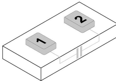
Figure 6 Pin configuration
