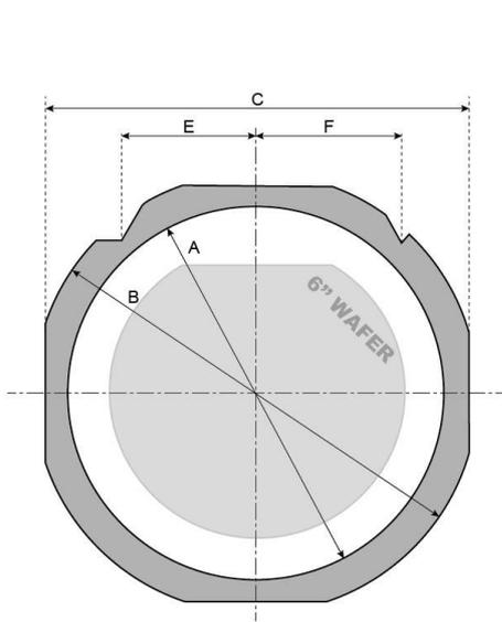
Figure 12 FF070 Frame with a 6" wafer
