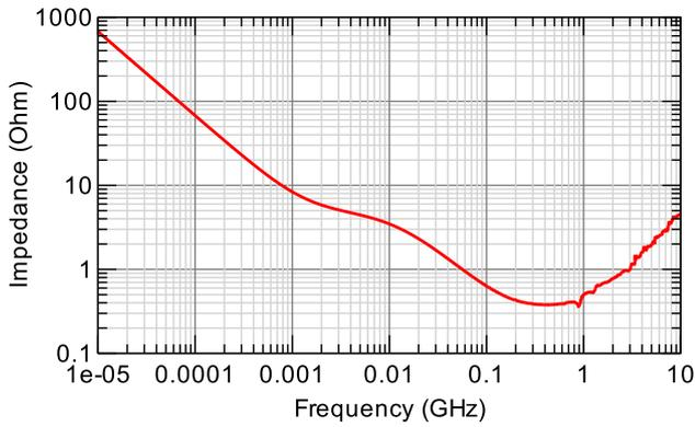
Figure 2 - 22nF ULSC Measured results (module of Z-parameters)
