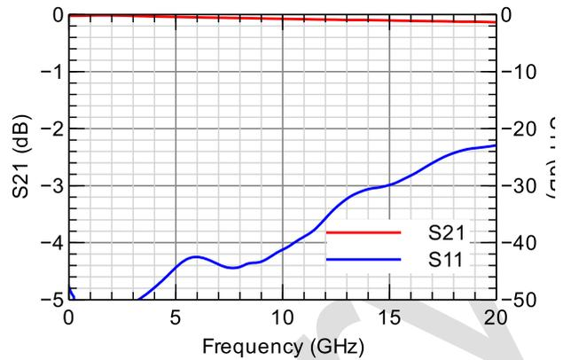
Figure 3 - 22nF ULSC measurement results (module of S-parameters)
