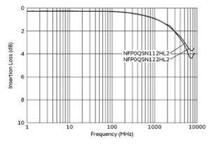
Differential Mode Transmission Characteristics (Typ.)
