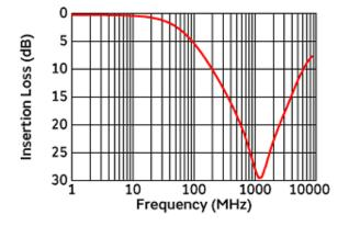
Common Mode Insertion Loss Characteristic(Typ.)
