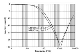
Common Mode Insertion Loss Characteristic (Main Items)(Typ.)
