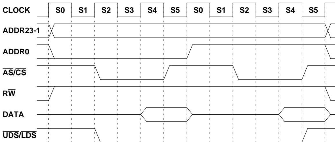
Figure 2-4. Word Read with 3-Clock 8-Bit Accesses
