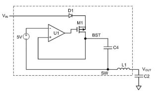
Figure 4: Internal Bootstrap Charging Circuit
