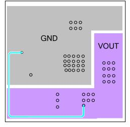
Bottom Layer Figure 7: Recommended PCB Layout
