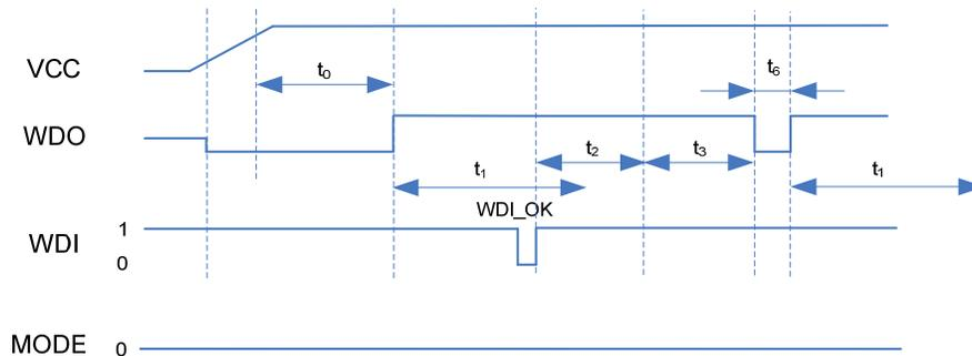
**Synchronized by WDI and triggered in closed window (MODE=0, short window mode)**
