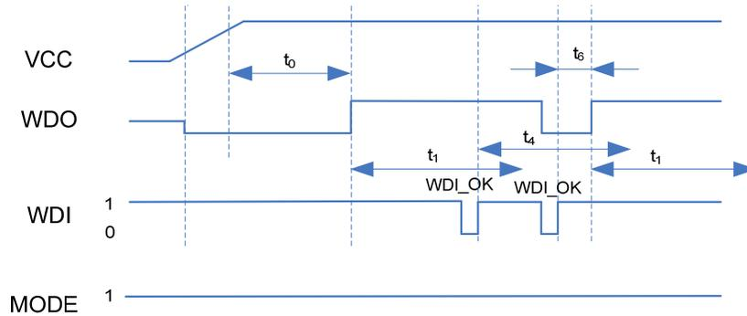
Note: When the WDI\_OK rising edge that comes at WDO is low, the  $t_6$  timer will be reset. Therefore, in the situation above, the WDO reset signal maintains a  $t_6 + \text{WDI\_OK}$  time.
