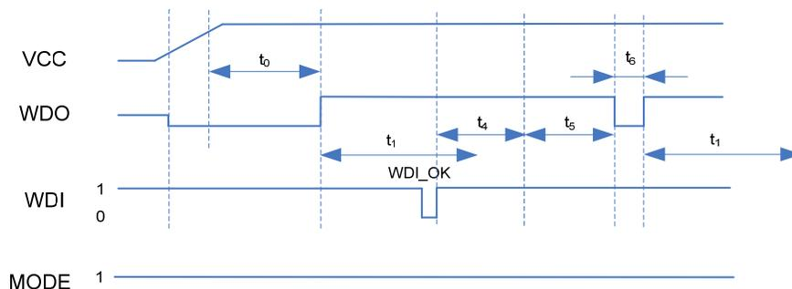
Synchronized by WDI and triggered in closed window (MODE=1, long window mode)
