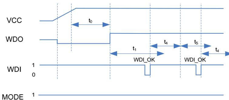
**Synchronized by WDI and no trigger signal (MODE=1, long window mode)**
