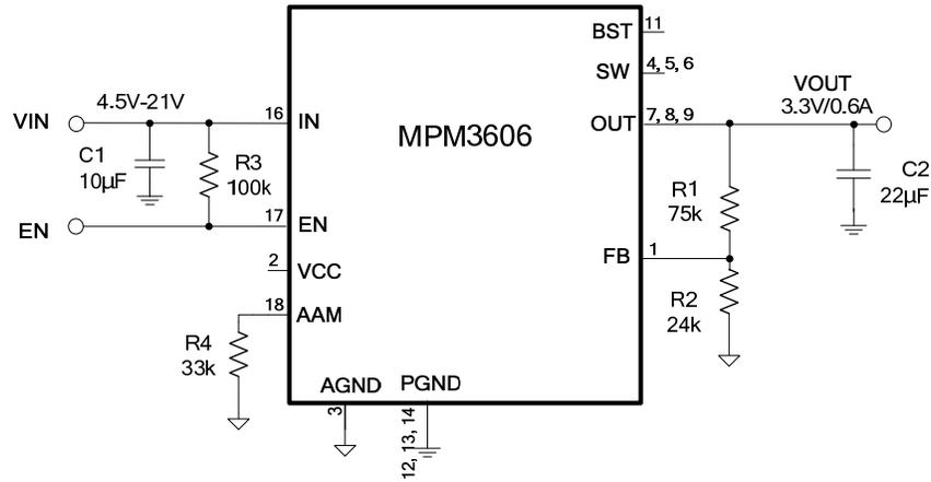
**Figure 9:  $V_{OUT}=3.3V$ ,  $I_{OUT}=0.6A$**
