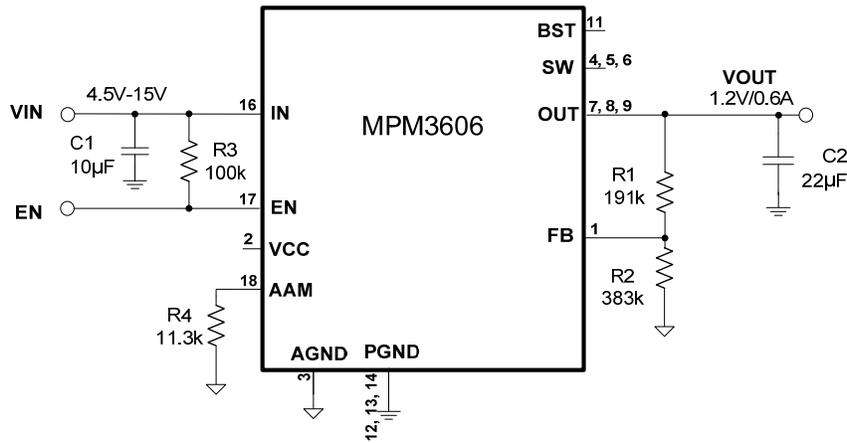
**Figure 12:  $V_{OUT}=1.2V$ ,  $I_{OUT}=0.6A$**
