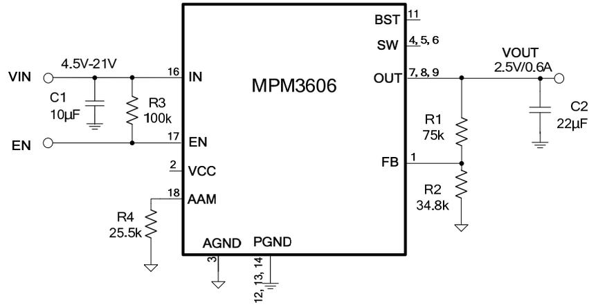
**Figure 10:  $V_{OUT}=2.5V$ ,  $I_{OUT}=0.6A$**
