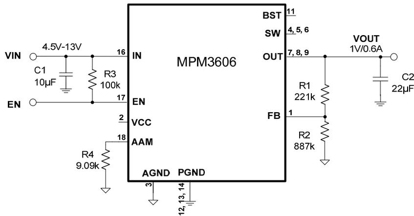
**Figure 13:  $V_{OUT}=1V$ ,  $I_{OUT}=0.6A$**
