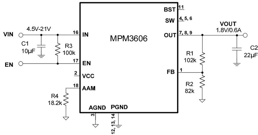
**Figure 11:  $V_{OUT}=1.8V$ ,  $I_{OUT}=0.6A$**
