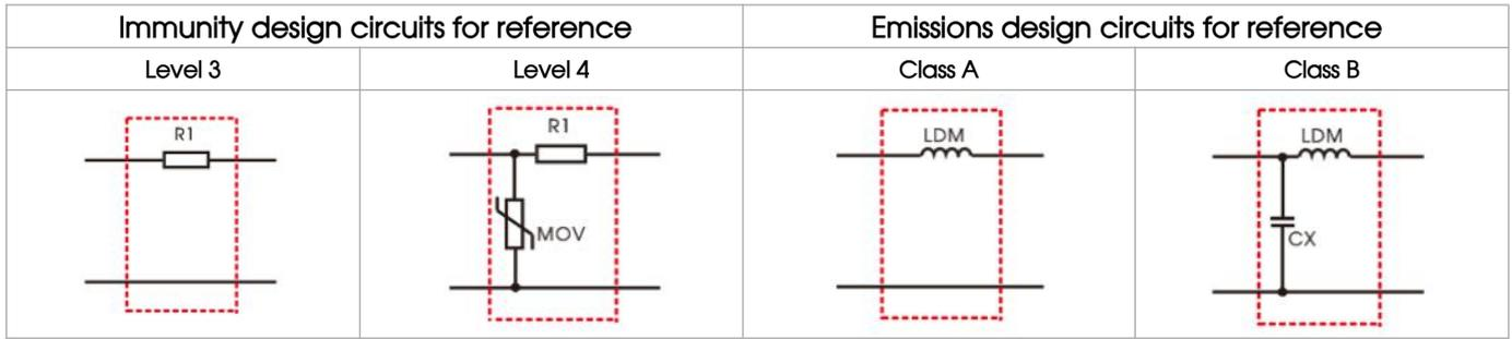
Electromagnetic Compatibility Solution--Recommended Circuit
