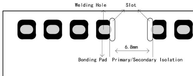
Note: There is a slot(non-metallic hole) between pin 4/5, which the side pad were being cut off. For details, please refer to the recommended dimensions or pad.
