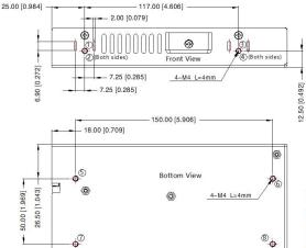
(1) – (8) any position must be connected to the earth( (4))
