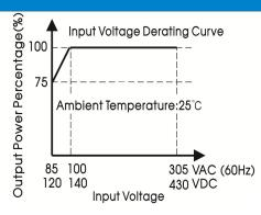
Note: 1. With an AC input voltage between 85-100VAC and a DC input between 120-140VDC, the output power must be derated as per the temperature derating curves;
