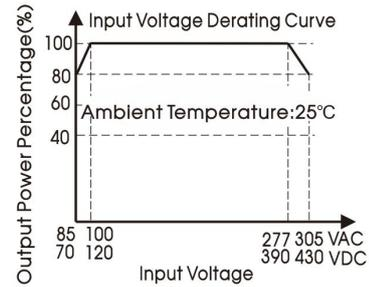
Note: ① With an AC input between 85-100VAC/277-305VAC and a DC input between 70-120VDC/390-430VDC, the output power must be derated as per temperature derating curves;
