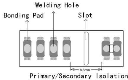
Note: There is a slot(non-metallic hole) between pin 4/5. For details, please refer to the recommended dimensions or pad.
