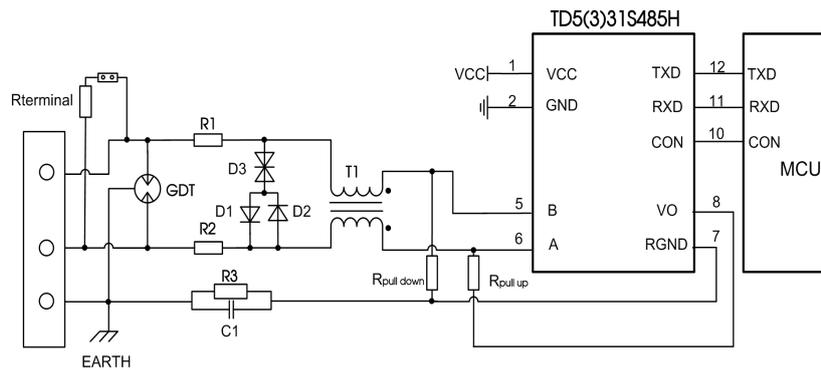
Fig. 2: Port protection circuit for harsh environments
