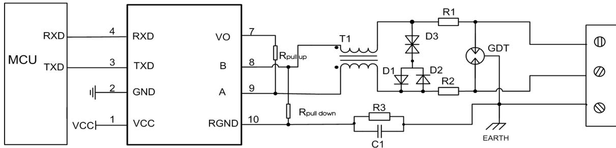
Fig. 2: Port protection circuit for harsh environments
