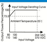
Note: 1. With an AC input voltage between 80-100VAC and a DC input between 110-140VDC the output power must be derated as per the temperature derating curves;
