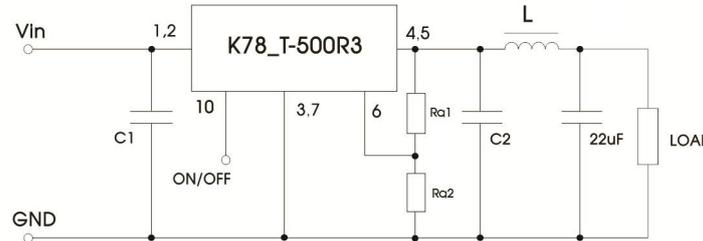
Fig. 3 External "LC" output filter circuit diagram
