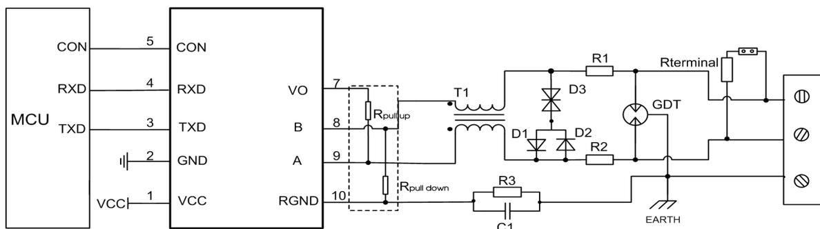
Fig. 2: Port protection circuit for harsh environments
