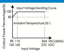
Note: 1. With an AC input voltage between 85-115VAC and a DC input between 120-160VDC the output power must be derated as per the temperature deratina curves,
