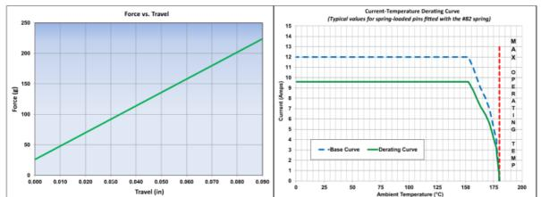
The stroke, force and current rating values are measured using spring pins with an internal construction per the design specification.
