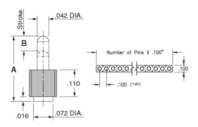
**Description:** Interconnect SLC Header Spring-Loaded Header Vertical Mount SMT Single Row Surface Mount **Plating Code:** Shell Plating: 20μ" Gold over 100μ" Nickel Inner Spring Plating: 10µ" Gold
