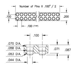
**Description:** Interconnect Flat Face Target Connector Spring-Loaded Header Vertical Mount SMT Target Double Row Surface Mount **Plating Code:** 10 Shell Plating: 10 µ" Gold over 100 µ" Nickel Packaging: Packaged in Bulk
