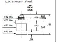
OPTO-X-5/-20-7X-14-11-0 Standard stroke, Surface mount Packaged on carrier tape. See chart for tape width and qty. per reel .042 DIA. .078 DIA. .070 DIA. .070 DIA. .072 DIA. Description:
