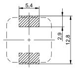
no sensitive traces underneath the component
