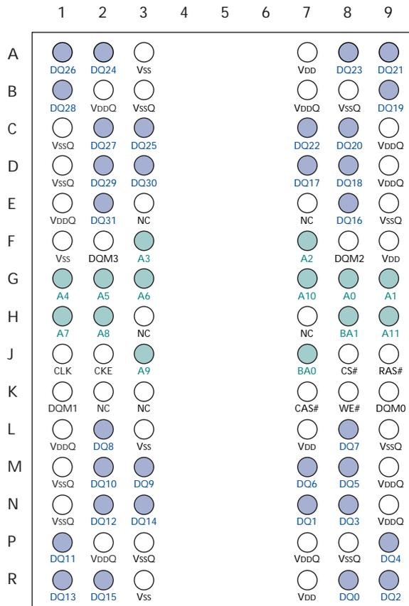
**Figure 5: 54-Pin TSOP Pin Assignment (Top View)**
