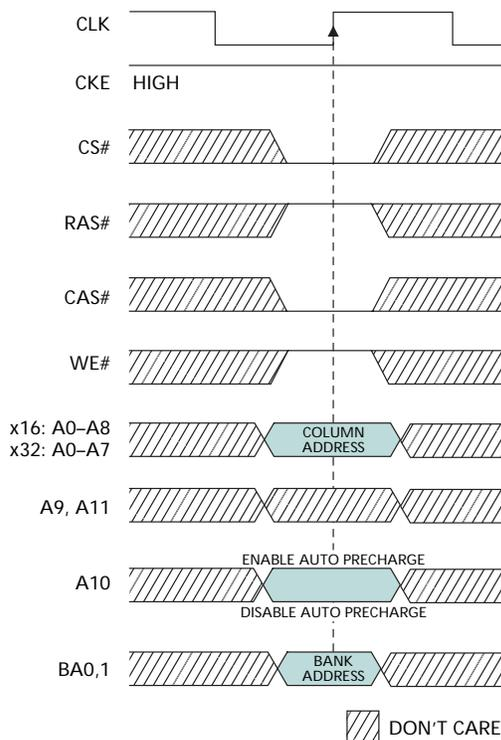
Upon completion of a burst, assuming no other commands have been initiated, the DQs will go High-Z. A full-page burst will continue until terminated. (At the end of the page, it will wrap to column 0 and continue.)
