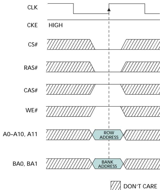
Figure 11: Example: Meeting  $t_{RCD} (MIN)$  When  $2 < t_{RCD} (MIN)/t_{CK} \leq 3$
