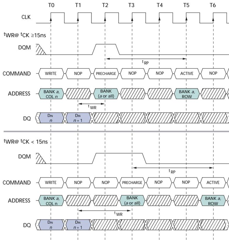
Notes: 1. DQM could remain LOW in this example if the WRITE burst is a fixed length of two.
