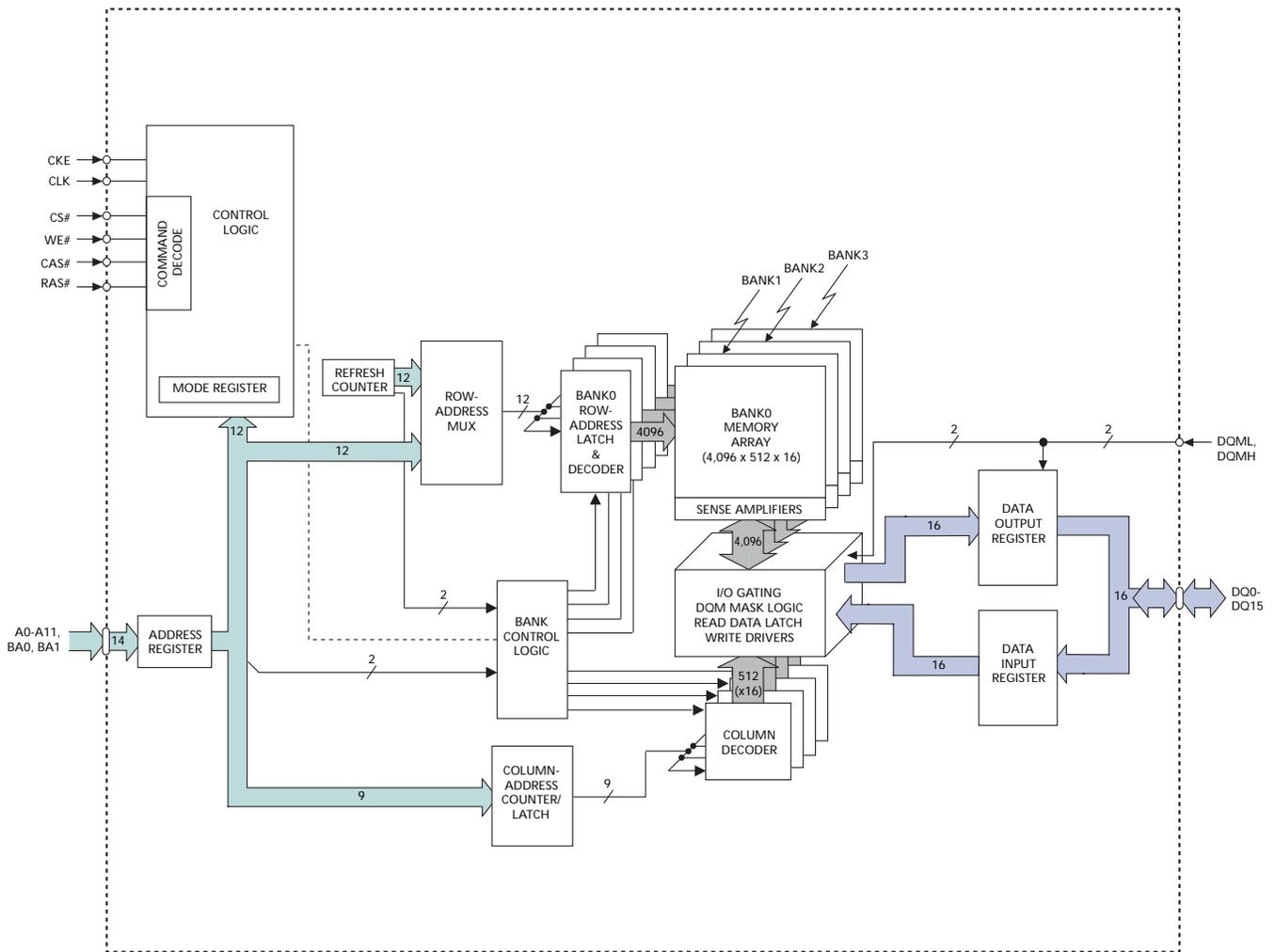
Figure 3: Functional Block Diagram 4 Meg x 32 SDRAM
