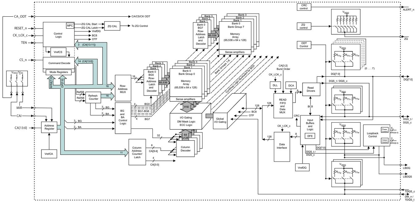
**Figure 4: 1 Gig x16 Functional Block Diagram**
