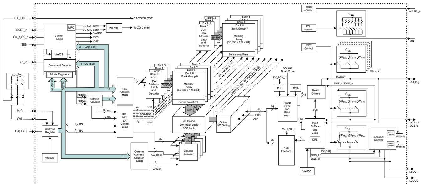
**Figure 3: 2 Gig x8 Functional Block Diagram**
